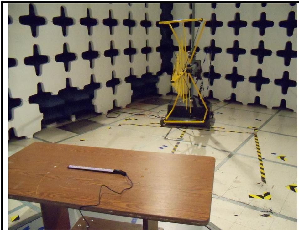
Test Setup Photo 2 – Radiated Emissions
