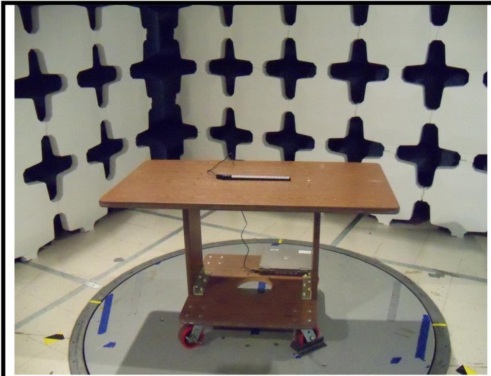
Test Setup Photo 1 – Radiated Emissions
