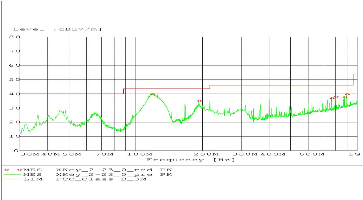
**Plot 3 – Radiated Emissions – 30MHz to 1GHz**
